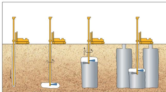
Fig. 1a Soilcrete® (drilling, cutting, soilcreting, extending)
