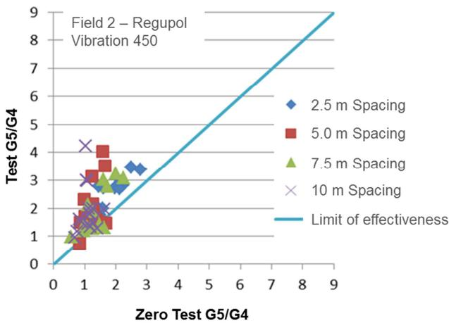
Fig. 8a Field 2 – Regupol Vibration 45
