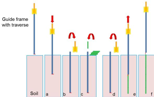
Fig. 4b Guide frame (left) and principle of the installation method (right)
