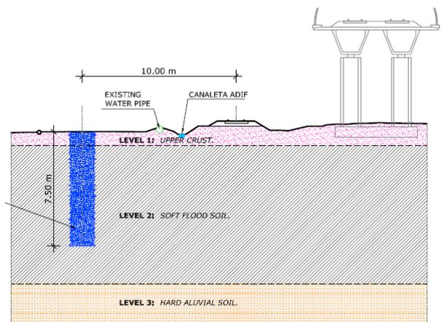
Fig. 3b Cross-section – Soilcrete® as a vertical wave barrier
