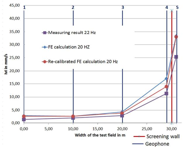
Fig. 11a Exemplary result of the recalculation – Field 1
