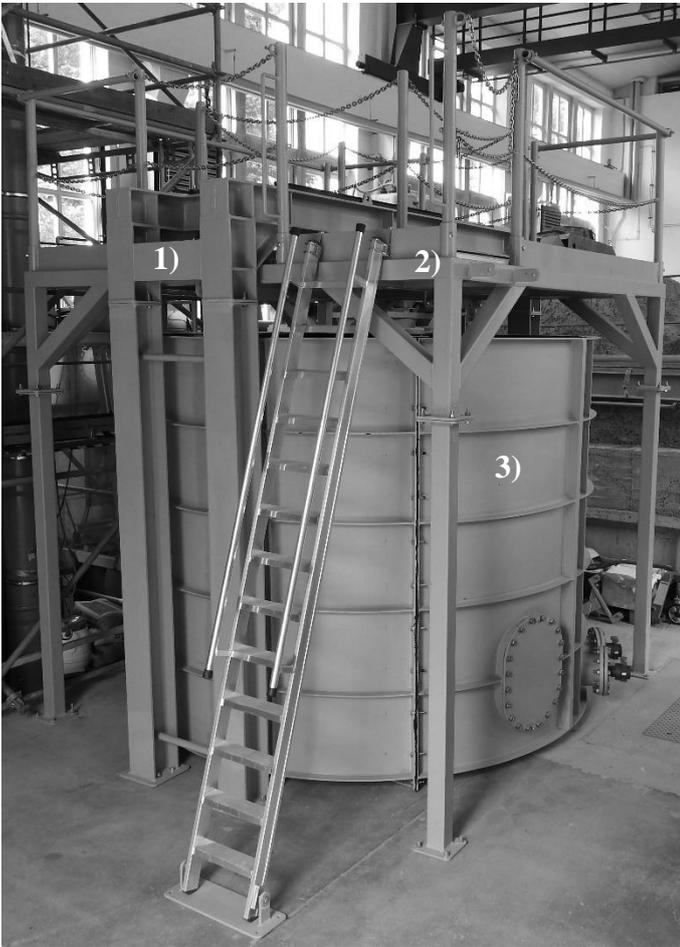
Figure 2. Pile test facility at TU Bergakademie Freiberg.
